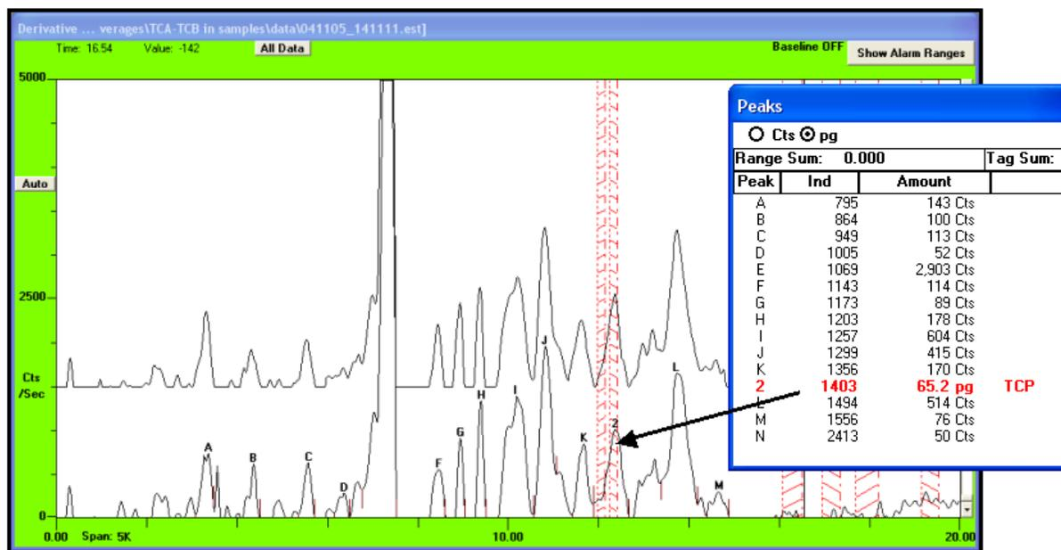
*Figure 8- Two vertically offset replicate chromatograms of headspace from wood samples heated to 40°C.*
