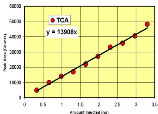
Figure 2- Direct injection of standards Figure 3- N-point calibration for TCA response
